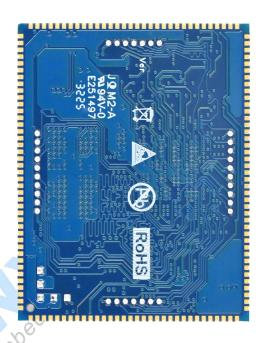
Note: PCB thickness is 1.2mm; total height of PCBA is 2.3mm; dimensional tolerance is  $\pm$  0.2mm.
